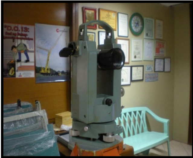
Surveyor's Transit on Tripod
